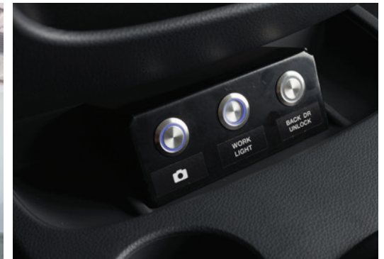
Control panel for locking and lighting system
