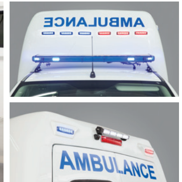
Emergency LED lights and LED emergency light bar
